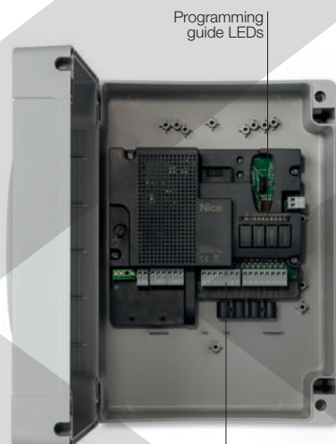
Removable terminals marked with connection codes
